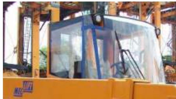
Figure 2-46: Damaged Windows at both MECLIFT Reach Stackers [Consultant]
